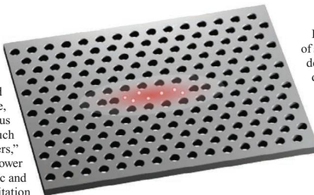
**Connecting the dots.** A high- $Q$  nanocavity (red) is formed in a 2D photonic-crystal slab that inhibits spontaneous emission. Quantum dots embedded in the nanocavity confine electrons (and holes) three-dimensionally and have sharp gain functions. Such a configuration may allow thresholdless laser operation.
